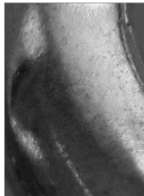
Figure 8 Lot 8, burnished in magnetic pin burnisher
