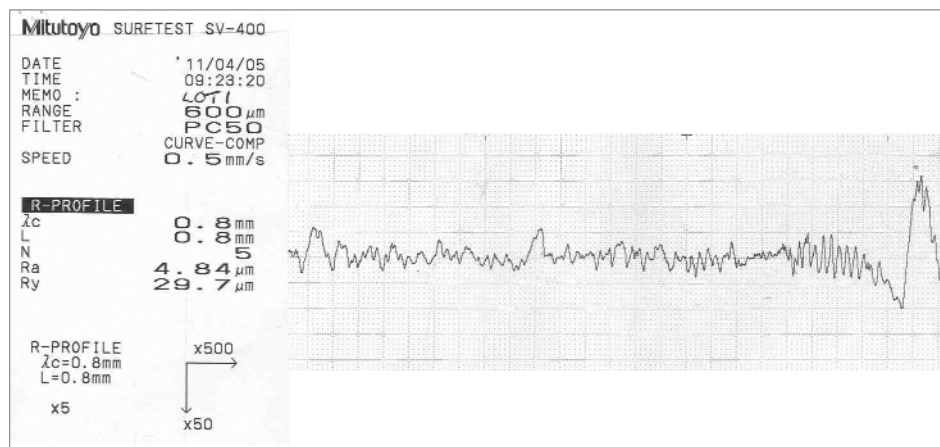
Figure 10 Surface profile chart, before burnishing
